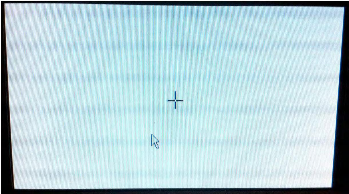
Touch the cross in the middle and then one more time in every corner and finally OK to calibrate the touch panel.
