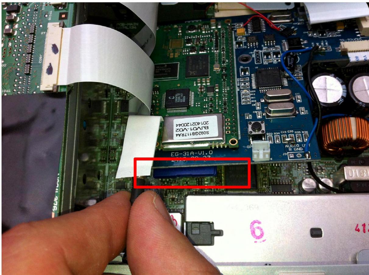
Tilt the PCB upwards slightly and you will be able to click the SD card out. It is in this area, on the bottom side of the PCB. It is not visible unless you click it out which I have done here.
