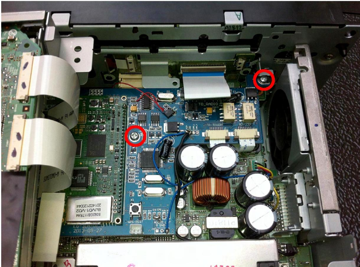
Tilt the DVD-drive over on the side and find two more screws you need to remove. Remove the two cables that hold the DVD-drive in place. They are visible as white straps on the left in this photo. Remove the DVD-drive completely and put it on the side for now.
