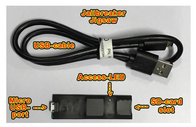
Make sure the SD-card is seated correctly in the SD-card slot.
