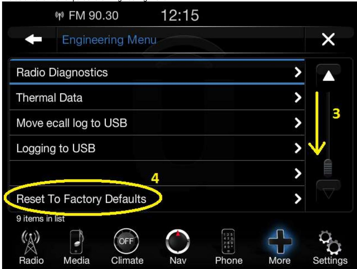
The best way to initialise a car after a factory reset is to remove the positive cable from the cars battery for 5 minutes.
